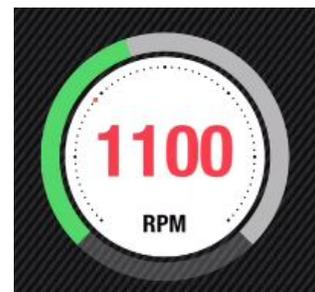
Below 800 RPM, the arc color is displayed Red (As a reminder that built-in alternator for equipped E-Mag module only start around 800 RPM and above.
