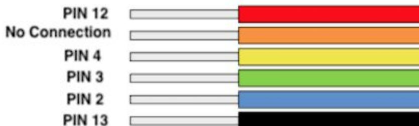
A Capacitor (included) needs to be soldered between the Red & Black. See Notes & Recommendations section of this manual.
