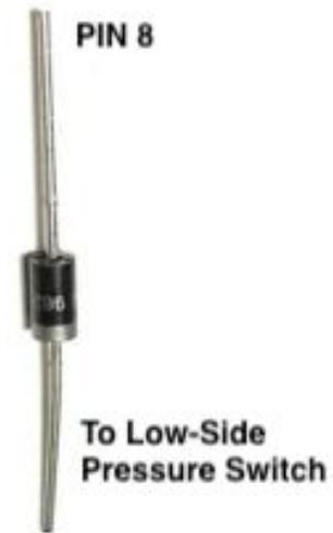
The Controller Switching Power module is capable of switching up to 3.5A, and this can be connected to a Power Switch that drives a mechanical solenoid which normally takes 2.5A. However, the Diode needs to be replaced with a 4A or higher Schottky Diode (not included)
