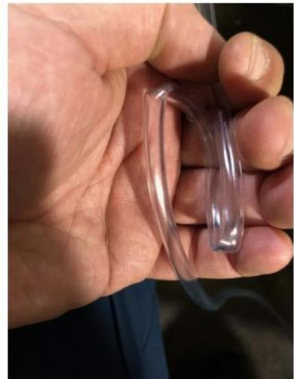
This method allows determining the required pressure to blow to get the speed up without damaging any installed sensitive pressure sensors. Squeeze more on the bends to block the tube if you want the speed to stop. Relax your hand slowly for the speed to decrease.
